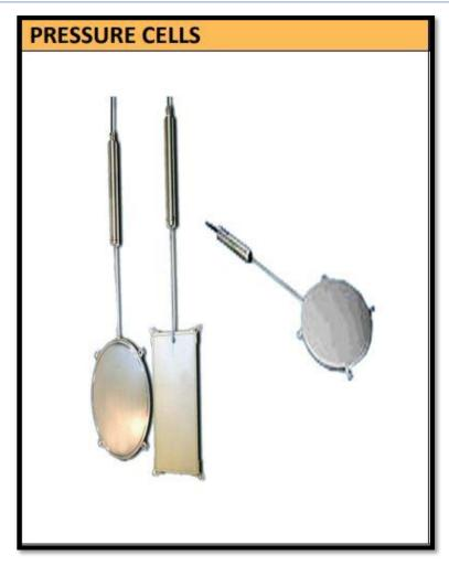
The Total Pressure Cell are used to measure total pressure in soils and embankments, at the interface of two different materials or measurements of stress in concrete. They are also used for measurement of contact pressures on retaining walls, buildings, bridge, abutments, tunnel lining etc.
