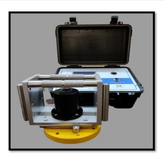
The Data Digger Equipment's model DDE-70M portable tilt meter is suitable for monitoring change in inclination of a structure. It is a high resolution tilt meter using the same proven technology as used in our inclinometer probe. It is rugged in construction and has excellent temperature stability. Tilt changes in structures may be caused due to construction activities such as excavation, tunnelling and dewatering that affects the ground that supports the structure.
