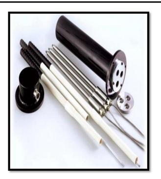
The DDE-7000 Series Borehole Extensometer Electrical/Mechanical (E/M), single or Multi-Point Borehole Extensometers are used to accurately measure longitudinal displacement in rock masses or concrete boreholes. It is particularly useful for distinguishing deep seated movements from surface spelling, which is of value in assessing the need for or determining the efficiency of a rock bolting system. The rugged low cost rod extensometer is designed to be easily installed in difficult locations.
