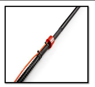
Data Digger's Equipment models DDE-5500RB Vibrating wire Re-bar strain gage, also known as Sister Bar strain gage, are specially designed for embedment in concrete structures. These are ideal for measurement of strain in concrete structures such as piles, diaphragm/slurry walls, bridge abutments, tunnel lining, dams, foundations etc.
