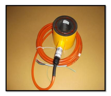
The Load Cell is designed to measure Unidirectional load in anchors and structural elements associated with many type of structures like:
