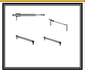
Model DDE -120 Crackmeter are used to measure movements across surface cracks or joints in structures, concrete or rock. The Crackmeter incorporates vibrating wire sensor with the resonant frequency of vibration of a tensioned steel wire is proportional to the strain or tension in the wire. This fundamental relationship is utilized in a variety of configurations for the measurement of load.
